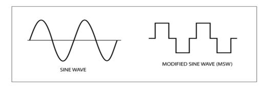
If you want to run your equipment exactly to the manufacturer's specifications, choose a pure sine wave inverter. With pure sine wave, motor loads start easier and run cooler. Some equipment only operate properly with pure sine wave inverter, such as laser printers, variable speed motors and digital clocks.
